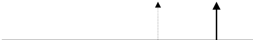
Figure 8-8. Interval Trigger that triggers when the interval falls within the selected range: T1=range's lower time limit; T2=range's upper limit. The broken upward pointing arrow indicates a potential trigger, while the bold one indicates where the actual trigger occurs — on the positive edge within the selected range.
