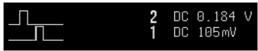
Figure 8-18. Qualified (top) and Qualified First (bottom) triggers compared: Whereas the (Edge-) Qualified Trigger requires that each of the segments be "qualified" by a valid condition in Sequence Mode, Qualified First Trigger needs only a single valid condition to qualify a full sequence of segments. Note that the inter-segment dead time (DT) is much shorter with Qualified First, which is used only in Sequence Mode. The display example shows Qualified First Trigger.
